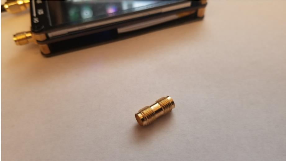
This is a calibration standard with the female to female adapter attached. These two are now a couple, a single item that will never again be separated:
