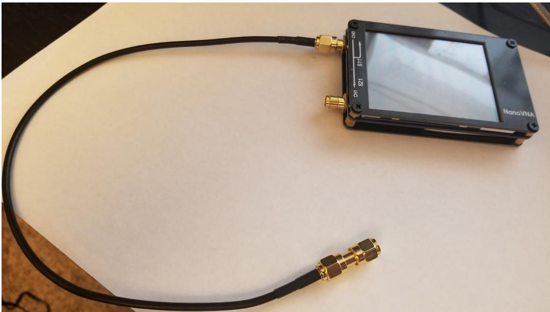
Now the calibration plane has been moved to the end of the coax. This arrangement is much more flexible – in several ways.
